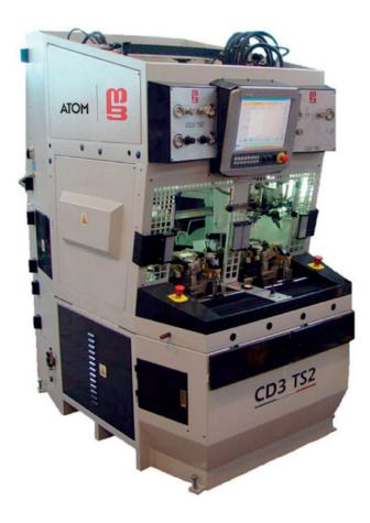
Roughing-cementing machine for the shoe bottom. The two operations are carried out simoultaneously thanks to two working heads, operating on two lasts carrier carts.
